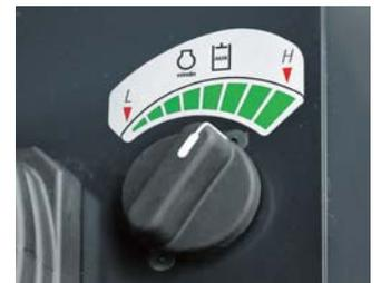
**Engine speed (AUX flow) control dial:**
