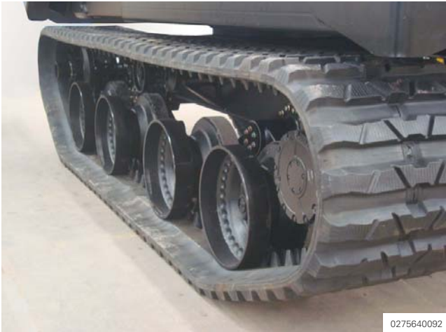
Figure 163 Normal track tension (generic Panther shown)
