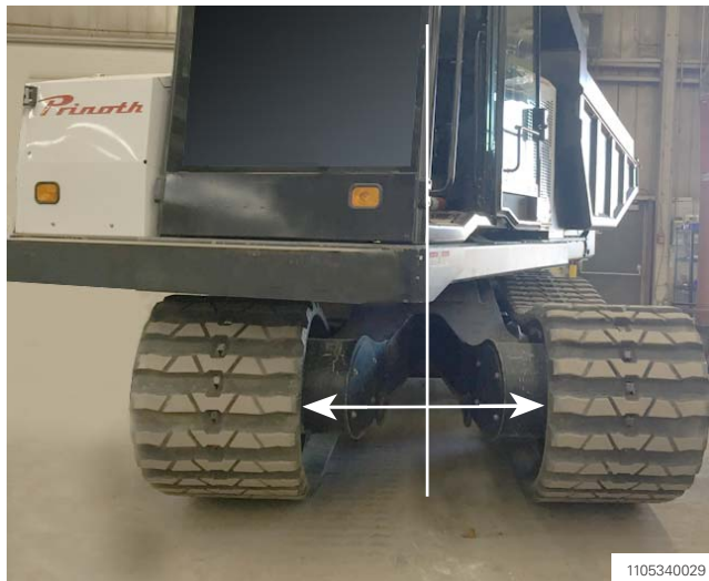
Figure 192 How to position the upper frame for the procedure
