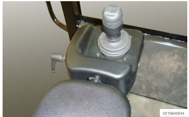
Figure 169 Joystick with swing function
