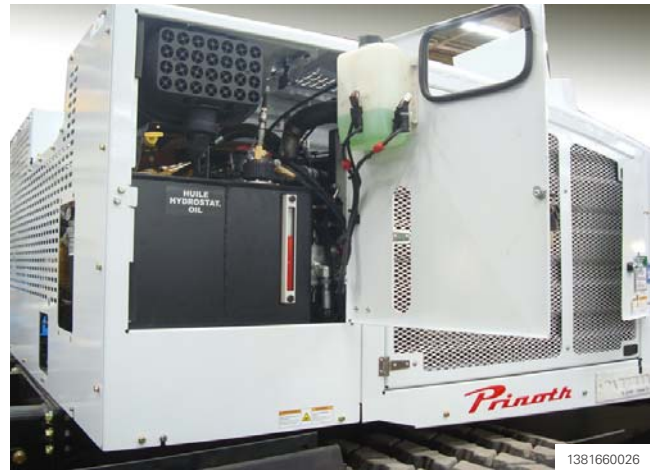
Figure 138 Lateral right side access panel (rear) - engine oil dipstick, oil tank filler neck and sight glass, engine air filter, windshield washer fluid tank and track tension release buttons (rubber track vehicle)
