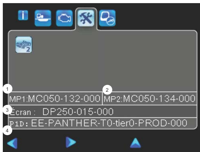
Figure 57 Microcontroller and display software part numbers 1. MP1, no of the main microcontroller software 2. MP2, no of the second microcontroller software 3. Display, no of the software 4. P1D, no of the software parameter
