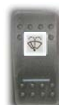
Figure 87 This switch controls the operation of the rear window wiper and washer fluid. Press the switch to the first stop to activate the wiper. Press the switch to the second stop (spring-load position) to activate the washer fluid pump.
