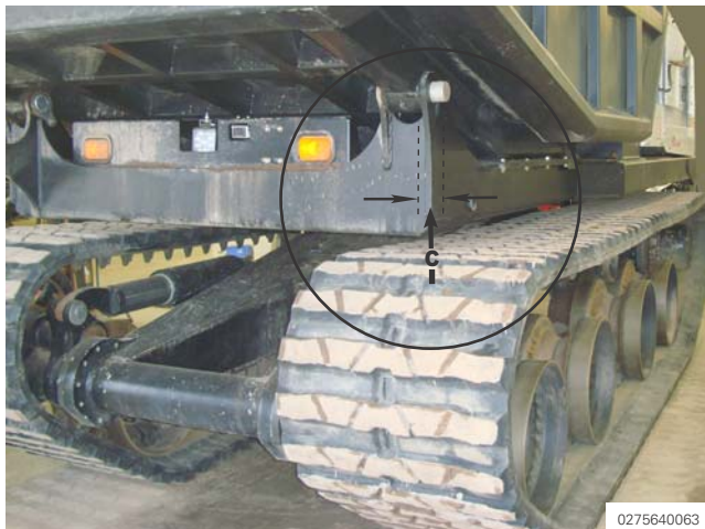
Figure 244 Backlash measurement location
