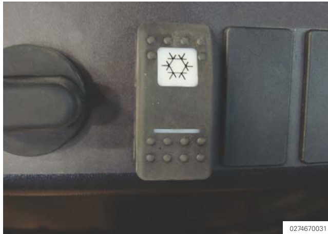
Figure 35 Air conditioning switch
