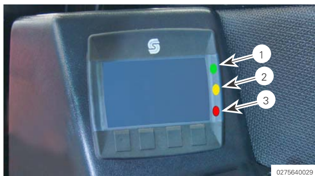
Figure 48 1. Upper frame is centered (green LED) 2. Joystick OFF (rotation and dumping are disabled - yellow LED) 3. Upper frame is inverted (transmission and steering are NOT inverted - red LED)
