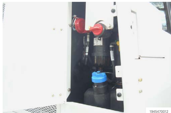
Figure 140 Lateral right side (front) access panel - DEF/AdBlue tank, water separator, secondary fuel filter and battery isolator switch.
