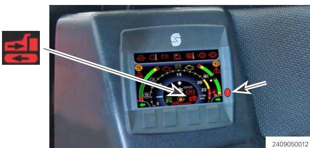
Figure 25 Inverted configuration icon and red LED on display right edge.
