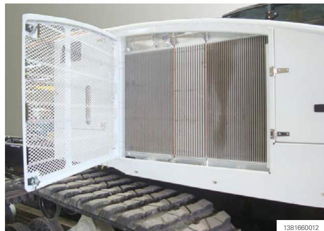
Figure 139 Center lateral right side access panel (access to radiators and cooler for cleaning)
