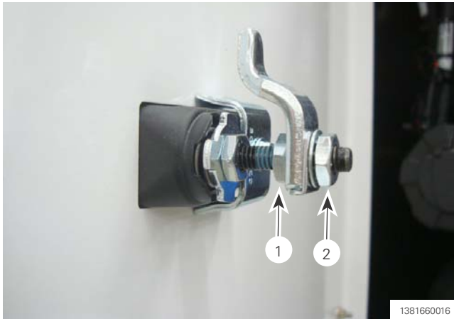
Figure 135 Access panel latch 1. Inner nut 2. Outer nut
