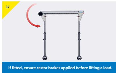
If fitted, ensure castor brakes applied before lifting a load.
