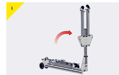
1 Rotate upper A-Frame to a vertical position.
